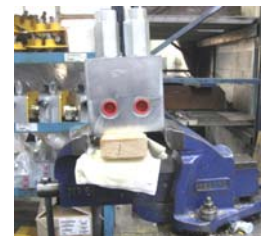
Figure 13: 2x4 used to mock up the preferred height of the vise
