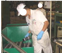
Figure 8: Mock up of loading parts into the first layer of the raised cart
