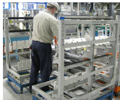
Figure 5: custom bin with walk-in floor
